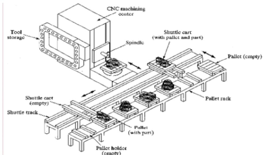
Fig 2.1: Single Machine Cell (SMC)
