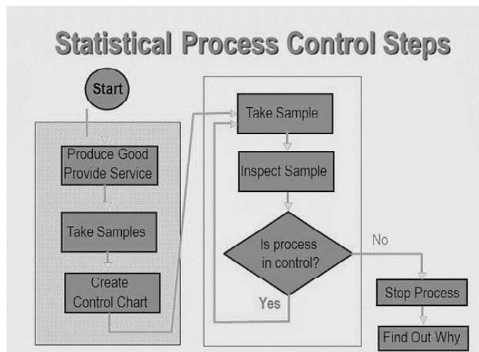
Fig 2.7: Statistical Process Control (SPC) Steps
